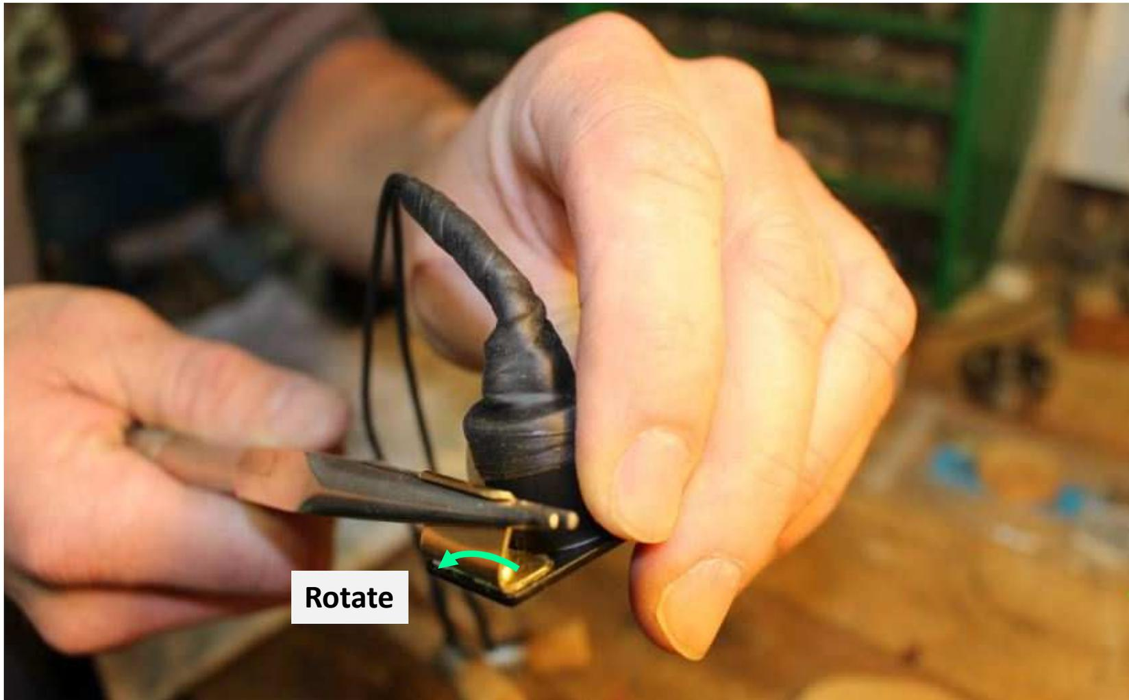
Before installation check the pickup cable orientation. It must be directed to the left when XLR pinout are down oriented, as shown on the picture.
