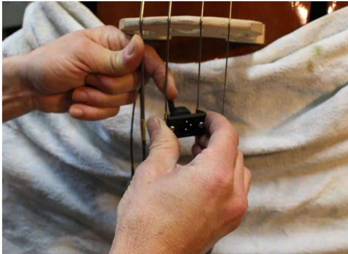
Example of standard connector installation. Remark connector spings do not force on A - D strings, which are still parallel.
