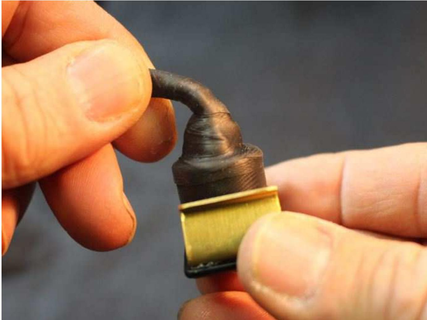
If cable angle is not good, position easy the cable base. Form a soft 90° angle carefully, using your 2 hands, to avoid any mechanical constraints on the cable base
